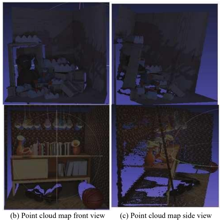
Figure 3: Network depth estimation map and its 3D reconstruction point cloud map on the HCINew dataset
