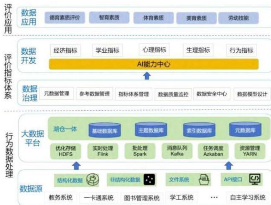
Figure 1: Architecture Diagram of the Student Comprehensive Evaluation System
